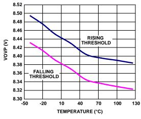
FIGURE 13. INPUT OVERVOLTAGE PROTECTION THRESHOLDS vs TEMPERATURE
