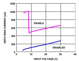
FIGURE 10. INPUT BIAS CURRENT vs INPUT VOLTAGE WHEN ENABLED AND DISABLED
