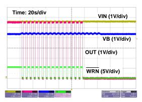
FIGURE 7. BATTERY OVERVOLTAGE PROTECTION. THE IC IS LATCHED OFF AFTER 16 COUNTS OF PROTECTION. VB VOLTAGE VARIES BETWEEN 4.3V TO 4.5V **Typical Operating Performance**The test conditions for the Typical Operating Performance are:  $V_{IN} = 5V$ ,  $T_A = +25^{\circ}C$ ,<br/> $R_{ILIM} = 25.5k\Omega$ ,  $R_{VB} = 200k\Omega$ , Unless Otherwise Noted. (Continued)
