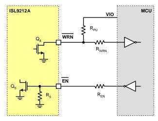
FIGURE 24. DIGITAL SIGNAL INTERFACE BETWEEN ISL9212A AND MCU
