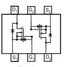
Top View Schematic and Transistor Diagram
