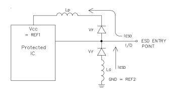
Figure 5 - The Effects of Parasitic Inductance
