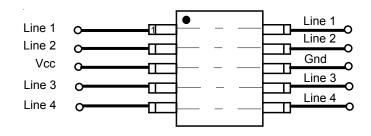
Figure 3. Data Line Protection Using Internal TVS
