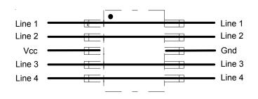
Figure 2. Data Line and Power Supply Protection Using Vcc as reference
