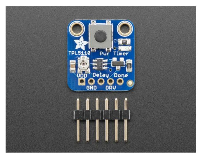
Usage is easy. First, set your desired delay but adjusting the on-board trim pot: all the way to the left is once-per-100ms an all the way to the right is once-every-2-hours. Then, connect VDD up to your 3-5V power supply and then your project's power-in to the Drive pin. Finally, select a signal pin from your project to the Done pin. In your project's code or design, just make sure that it sets the Done pin high once it is completed with it's task. That's it!
