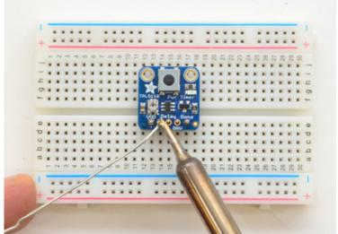
Be sure to solder all 5 pins for reliable electrical contact.
