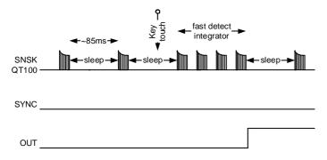
Figure 2.2 Fast Mode Bursts (SYNC held high)
