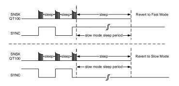
Figure 2.4 SYNC Mode (Short Pulses)
