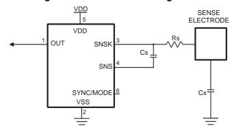
Note: A bypass capacitor should be tightly wired between Vdd and Vss and kept close to QT100 pin 5.
