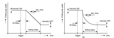
Figure 28 GPO OFF transition (LED fade out), normal polarity, (a) linear, (b) logarithmic
