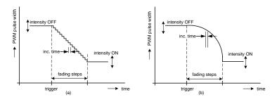
Figure 27 GPO ON transition (LED fade in), inverted polarity, (a) linear, (b) logarithmic
