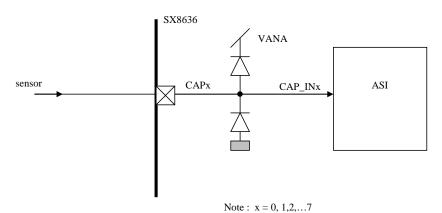
Figure 30 Simplified diagram of CAP0, CAP1, ..., CAP7
