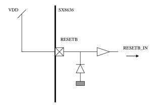
Figure 36 Simplified diagram of RESETB without host control
