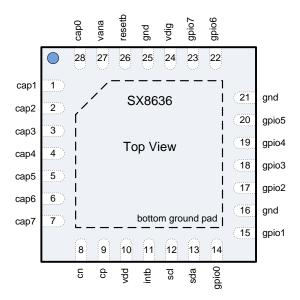
Figure 1 Pinout Diagram
