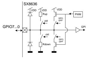
Figure 40 Simplified diagram of GPIO pins
