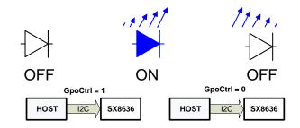
Figure 24 LED Control in GPO mode, Autolight OFF
