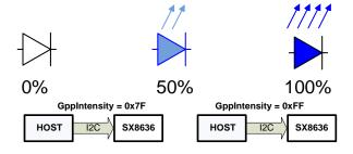
Figure 23 LED control in GPP mode
