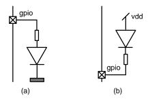
Figure 21 Polarity definition, (a) normal, (b) inverted
