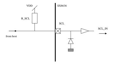
Figure 33 Simplified diagram of SCL
