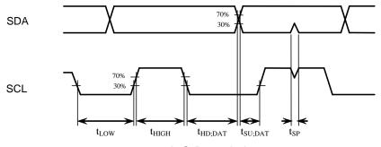
Figure 5 I2C Data timing
