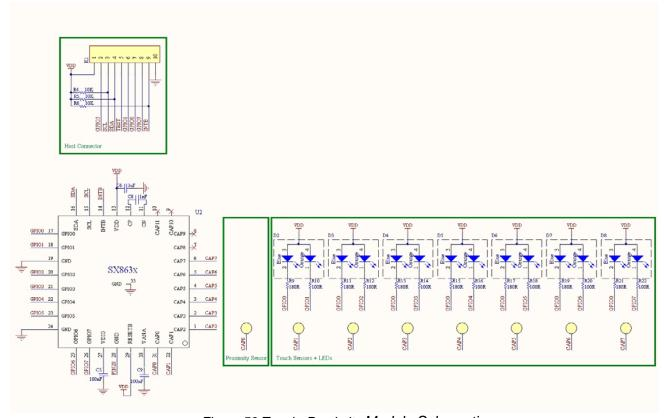
Figure 53 Touch+Proximity Module Schematics
