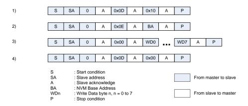
Figure 46: SPM Write Sequence
