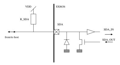
Figure 34 Simplified diagram of SDA
