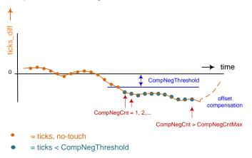
Figure 43 Negative Ticks Offset Compensation Trigger
