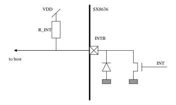
Figure 32 Simplified diagram of INTB
