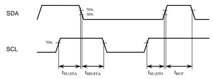
Figure 4 I2C Start and Stop timing
