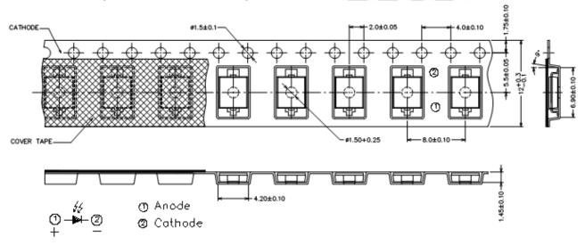
Note: The tolerances unless mentioned are ±0.1, unit=mm.
